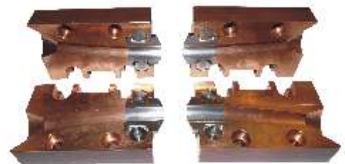
Series SS vertical clamping jaws for welding in the radius
